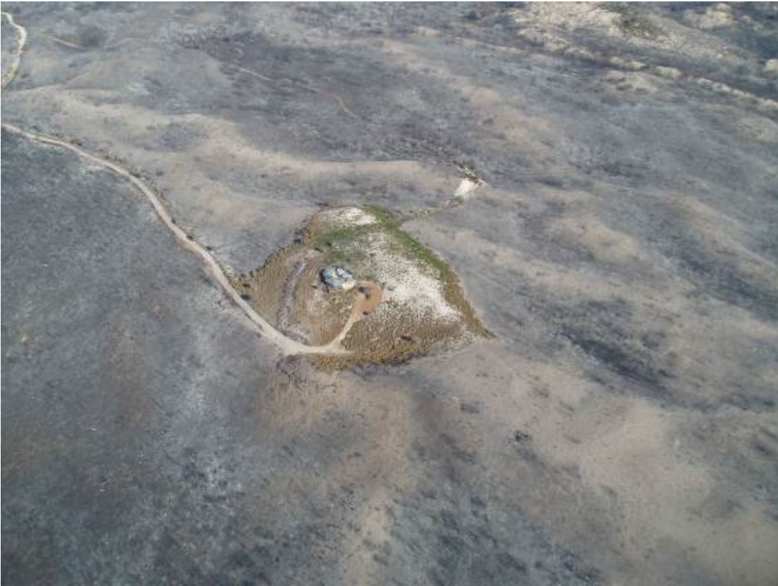
(Above and below). An isolated house during the Margaret River bushfires in November, 2011. It was saved as there was a perimeter sprinkler system which was automatically activated by heat.
